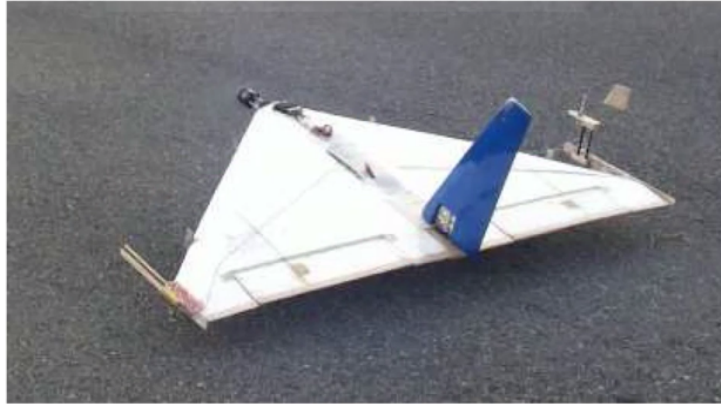
Wing cross section : Reflex Airfoil Wing planform : Cropped Delta Wing UAV Lab, Department of Aerospace Engineering, IIT Kanpur.
