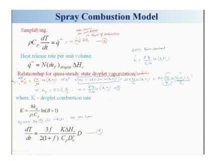
So, you can also write it down simplifying this, I can write down rho Cp dT by dt is equal to q dot triple dash and this is equal to N m dot f into delta HC number density that number of droplets and this is this is basically mass consumption right, mass burning per unit droplet right into delta HC is the heat of combustion, this is basically heat of combustion right.
