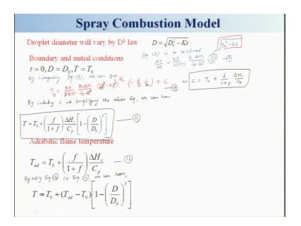
So, therefore, we can write or droplet diameter will vary by D square law that is D is equal to D 0 square minus Kt and the boundary and initial condition will be basically t is equal to 0 D is equal to D 0 and T is equal to T 0 right and like what we will do we will have to equation 9, we need to solve equation 9 is to be solved right, that is dT by dt temperature with respect to time is equal to 3 f 2 f plus 1 K delta HC by Cp D 0 q into D right
