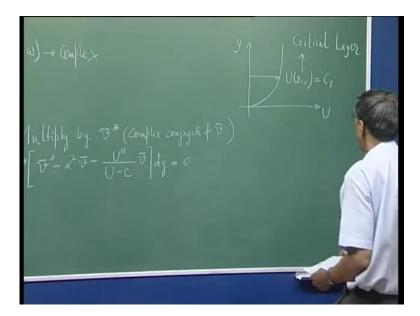
So, for a neutrally stable flow, you will have a height where this can match. What are we talking about? You see basically we are talking about the following that if I plot U versus y, then I could get a profile like this. So, at each height, I have a value of u. At some
