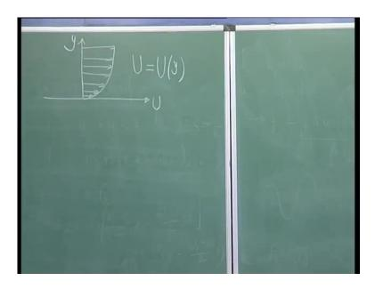
Basically, we can study the flow field which has this detailed variation of the velocity profile, given like this. So at different height I am going to get this kind of velocity distribution, and what is the characteristic of this velocity distribution that it maintains a shear. So the mean flow now has a shear, whereas what we studied before; zero shear case. So that is what I said that we are going to retch it up the difficulty of the description of the equilibrium flow.
