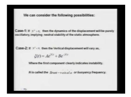
So, this expression, this was done by two Scandinavian scientists and this N is called the Brunt-Vaisala or buoyancy frequency, because it comes out in a simple harmonic motion a square. So, it has the dimension of a frequency. That is what you get for your simple harmonic motion of a pendulum. So, that is why N is called a frequency or the Brunt-Vaisala frequency.
