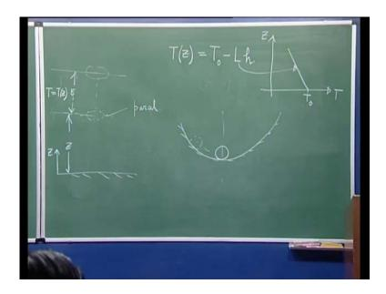
So, we can do a similar study actually. If I disturb it from here to here and let us say if I call this variation of temperature as given by T 0 minus say some height h, I am calling it, that is, its linearly falling. So, basically what we are talking about this T if I plot the height versus T, so its start off with some value T 0, and then, it is falling off like this. This rate at which it is falling is given by L.
