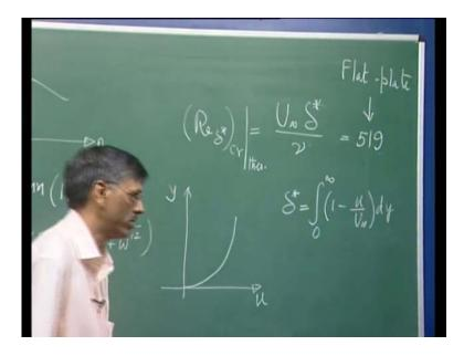
So, this Re critical that here, we are talking that this is experimental, and this is what we are defining here; this is a theoretical. So, this is like your transfer function telling you that the flow is ready. If Re delta star is 520, the flow is ready to become critical. If you provide the disturbance, it would show the signature of those disturbances.
