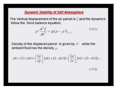
So, if I now talk about a unit volume, then its mass is rho prime and we have moved it vertically and it is going to experience a vertical force due to buoyancy. So, if I want to study its dynamics, I will write down this. So, this is mass times acceleration on the left hand side, and what is a buoyancy force? g times rho minus rho prime and this is where we are trying to find out at the disturbed location. The disturbed location is z plus xi.
