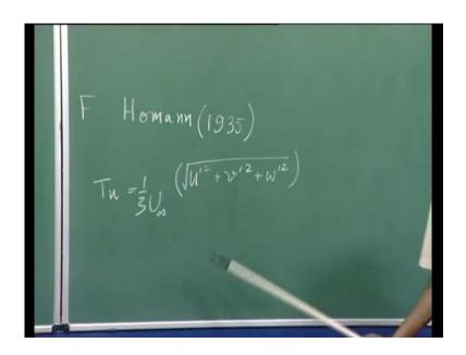
Turbulent intensity is defined as the following that, if we have a uniform flow infinity and then you measure the disturbance quantities, and if these are u prime, b prime, w prime, you look at it and that is your turbulent intensity. So, it is a basically nondimensional RMS fluctuation of the flow field.
