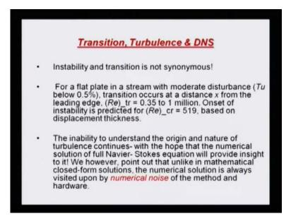
So, if you keep that turbulent intensity less than 0.5 percent, that means 0.005 or lower, then transition occurs at a distance x from the leading edge which is given about 350
