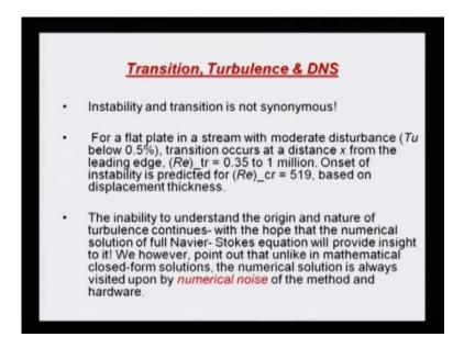
This is one thing that to we discussed earlier also that instability and transition is not synonymous, they do not occur in the same place. You may have a transitional flow. For example, if you look at a flat plate in a flow with moderate disturbance where, that turbulent density is less than 0.5. What is turbulent intensity?
