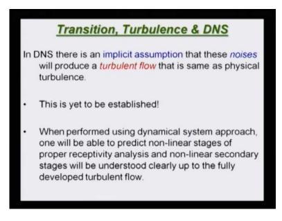
So, this is something we should keep in mind and that is what is being said in the next transparency that, when we are doing the simulation of Navier-Stokes equation without any modeling. So, we are solving the full Navier-Stokes equation without any models. That is what is called as direct numerical simulation or DNS.
