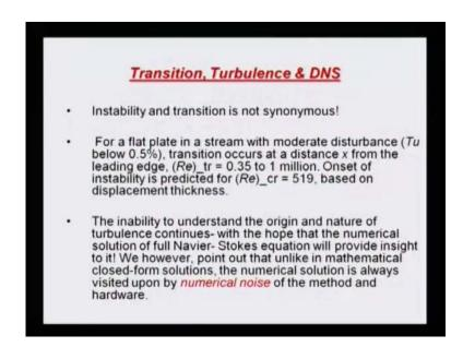
However, I would like to or we should point out that unlike in mathematical closed-form solution, numerical solution is always contaminated by noise. So, whatever we are saying here, the variability of the transaction point and the criticality depending on disturbance, that also may affect the Navier-Stokes solution.
