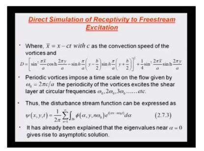
So, this is the way to ((run)) visualize the problem, that I would write down the disturbance stream function, which will be function of x, y and t; x of course, dependence can be figured out here, in terms of the phase i alpha x; alpha itself could be complex, because, we are applied it, talking about instability problem. What about the time dependence? Time dependence is going to be happening at omega naught, and its various harmonics.
