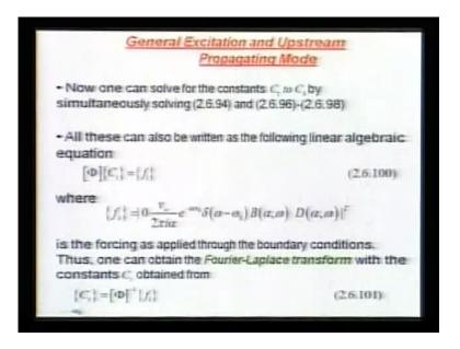
Now, then this completes that description of the boundary condition that will enable to really fix this constant C matrix, that would be given in terms of a 4 by 4 matrix, operating on the unknown constants is equal to the excitation. So, whatever may be the excitation that is put in on the right hand side. What is important, though that if this excitations are non-null, the non-zero, then what we can do is basically I can obtain this C i vector is equal to phi inverse of this.
