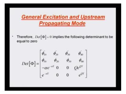
So, now, if we decide to look for those kind of modes for which real alpha is positive negative and real Q is positive then phi 2, and phi 3 are the decaying modes, and this 2 entries will go to 0, when y goes to infinity is a subdominant quantity, because we have e to the power plus alpha y so alpha r is positive.
