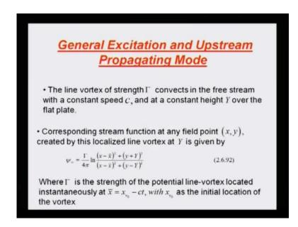
Now, what happens to this additional exciter in the free stream, and that is what we have started discussing over the last few lectures, and what we saw that the existence of that line vortex of strength gamma moving at a constant speed C at a constant height at Y gives rise to kind of a disturbance stream function, and this disturbance stream function provides a kind of a free stream in excitation.
