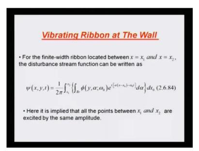
Suppose disturbance source is located at x equal to x naught, then this will be the solution, and again I can substitute it in linearized Navier stokes equation or apply a parallel flow approximation, so and, behold I get back the Orr-Somerfield equation for this phi, so for any point this is the governing equation remains the same, what I need to do is, that take that unit solution, where the exciter is at x naught, and then integrate over if range of x naught going from x 1 to x 2.
